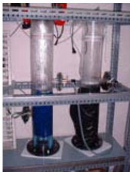
Fig. 1 Denitrification reactor (left) and nitrification reactor (right)
