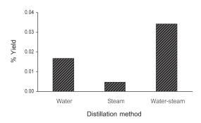
Figure 1 Comparison of the extraction yields of frangipani oil by distillation method.
