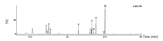
Figure 3 Chromatogram of essential oil from steam distillation.
