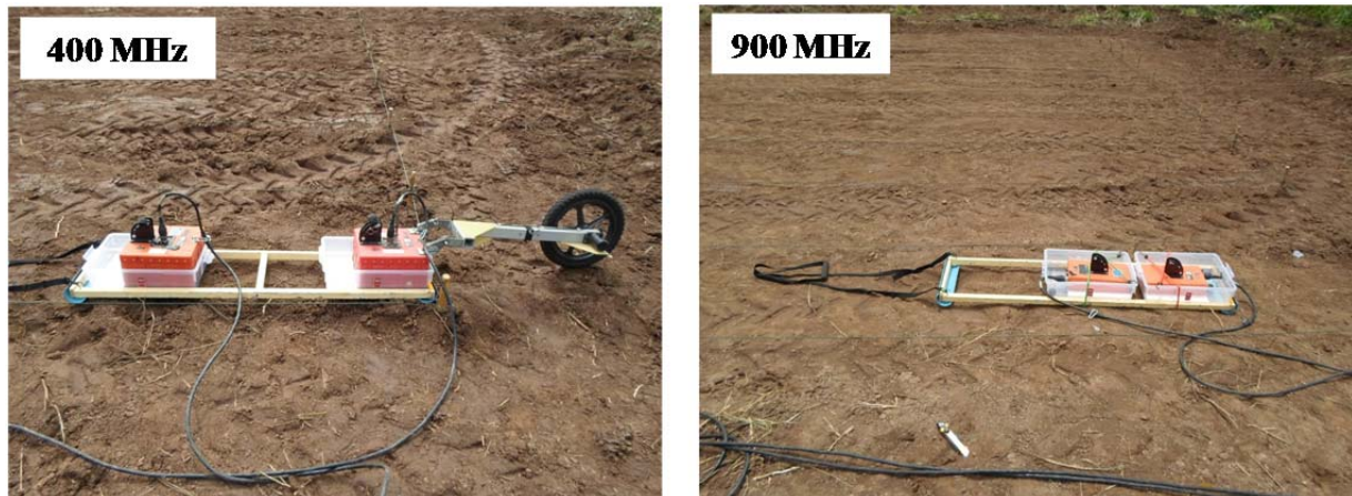
Figure 4 Sledge setup for the 400 MHz GPR (Left) and 900 MHz GPR (Right) survey systems
