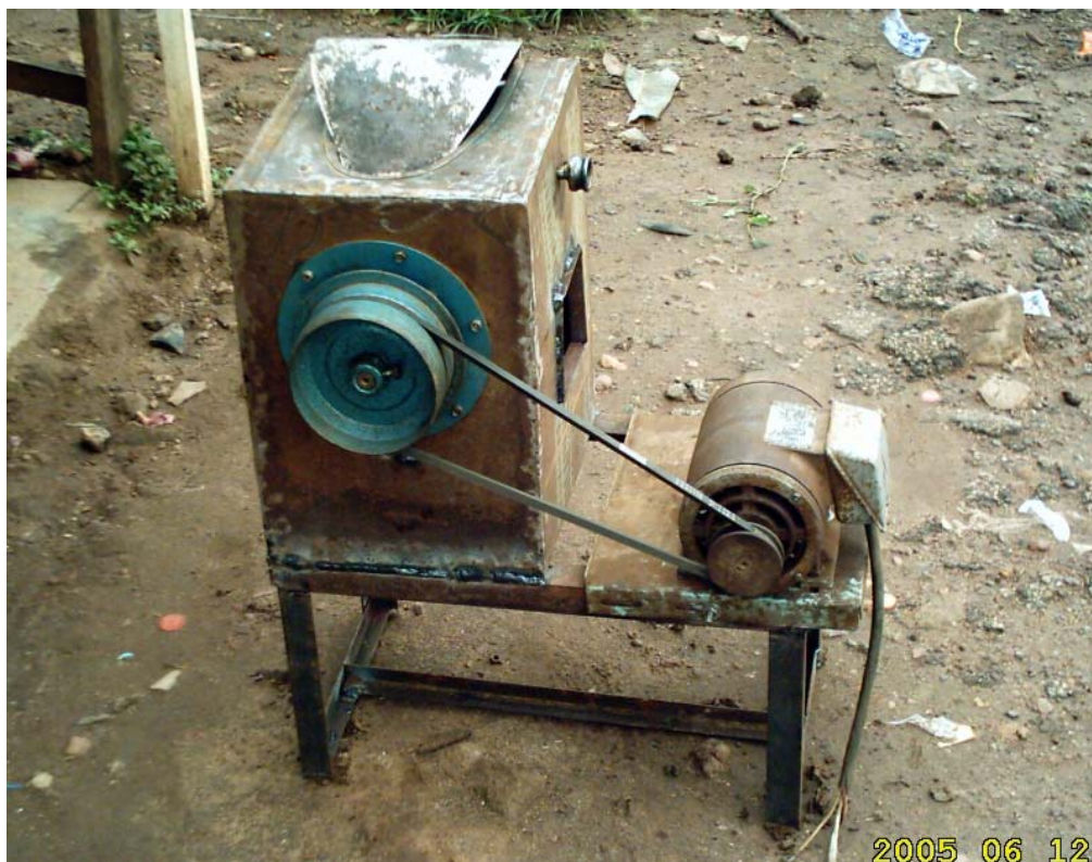
Fig. 5. Plate 2 - Back view of the machine showing the belt and the electric motor.
