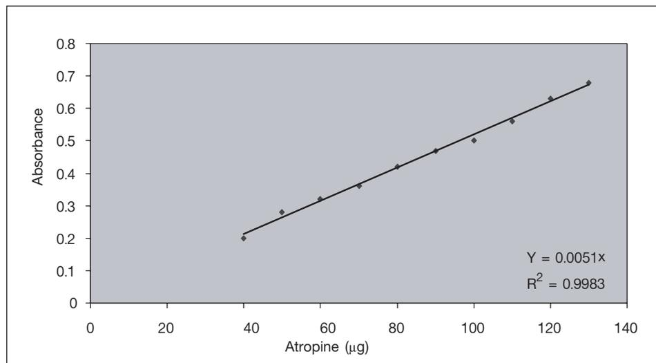
**Figure 1** Variation of the absorbance with atropine concentrations at 470 nm
