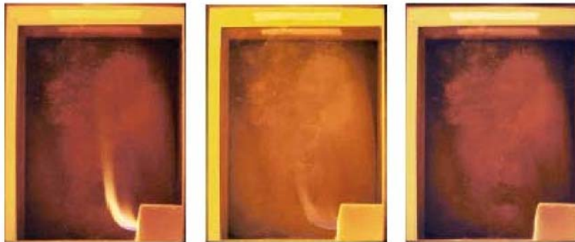
Figure 11 (a). Hydrogen flame photographs with combustion air temperature of 1000°C and oxygen concentrations (from left to right) of 21%, 8% and 2%, respectively (nitrogen as the dilution gas).
