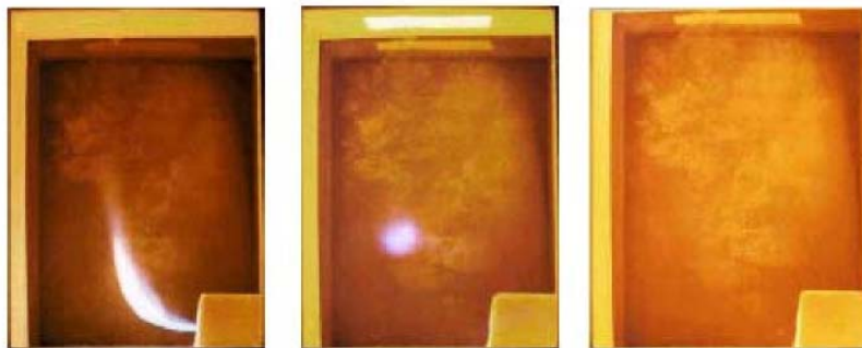
Figure 10 (a). Methane flame photographs with combustion air temperature of 1000°C and oxygen concentrations (from left to right) of 21%, 8% and 2%, respectively (nitrogen as the dilution gas).
