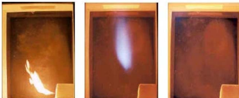
Figure 12(b). Acetylene flame photographs with combustion air temperature of 1000°C and oxygen concentrations (from left to right) of 21%, 8% and 2%, respectively (carbon dioxide as the dilution gas).
