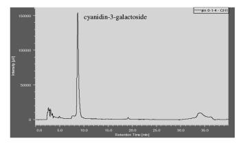
Figure 1. HPLC chromatogram of anthocyanin in the ethanolic extract of *Carissa carandas*.
