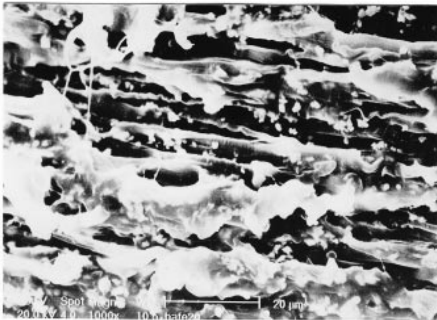
Figure 5e : SEM micrograph for fractured 4 vol.% TPNR composite
