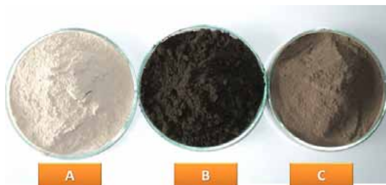
Figure 3. The features of fresh bleaching earth (A), Spent bleaching earth (B), and Reactivated bleaching earth (C)
