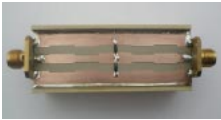
Fig. 4 The completed insertion type CBCPW phase shifter on the RO3006 microwave substrate with two shunted-varactors.
