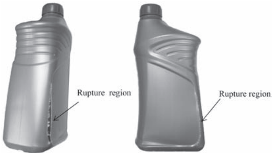
Figure 7 Ruptures found on the side of the HDPE bottles after the drop impact test.
