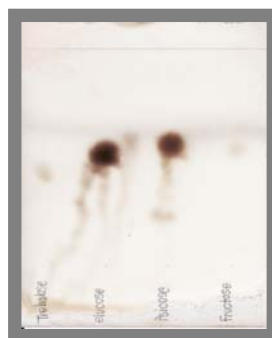
Figure 2. Chromatogram of standard sugar by spraying with 20% H 2 SO 4
