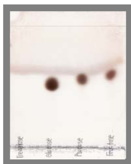
Figure 1. Chromatogram of standard sugar by spraying with methanol : H 2 SO 4 (1:1)
