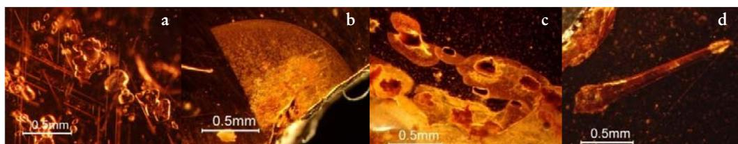
**Figure 3.** Showing typical inclusions in Thai pyrope garnets: (a) needles and crystals (BK 05), (b) liquid inclusion (KW 51), (c) tension discs (NB 25) and (d) hollow tube (KW 34) (darkfilled illumination).
