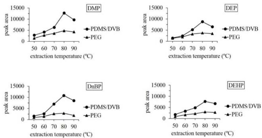
**Figure 1.** Effect of extraction temperature on HS-SPME of spiked 200 ng mL<sup>-1</sup> of four phthalate esters in vegetable oil sample with extraction time of 30 min, desorption time of 10 min at 200 °C.
