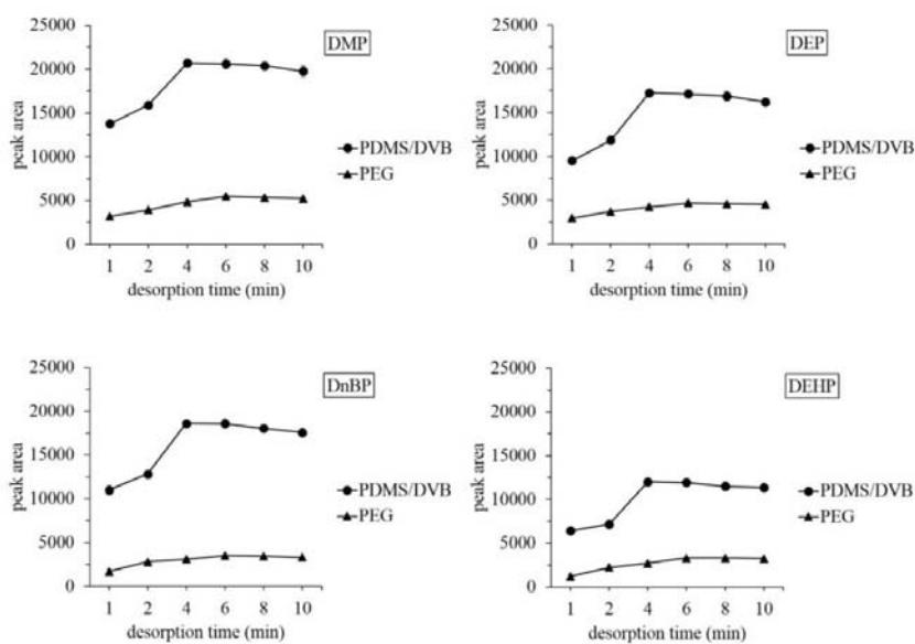
**Figure 3.** Effect of desorption time on HS-SPME of spiked 200 ng mL<sup>-1</sup> of four phthalate esters in vegetable oil sample with extraction temperature of 80 °C, extraction time of 30 min and desorption temperature of 200 °C.
