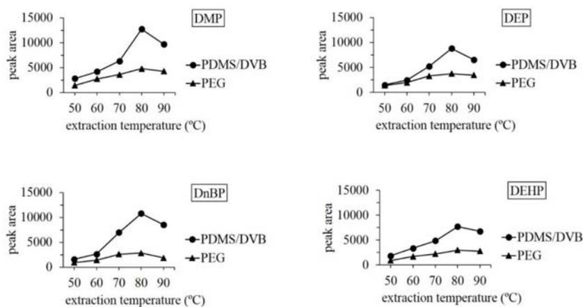
**Figure 1.** Effect of extraction temperature on HS-SPME of spiked  $200 \text{ ng mL}^{-1}$  of four phthalate esters in vegetable oil sample with extraction time of 30 min, desorption time of 10 min at  $200 \text{ }^{\circ}\text{C}$ .
