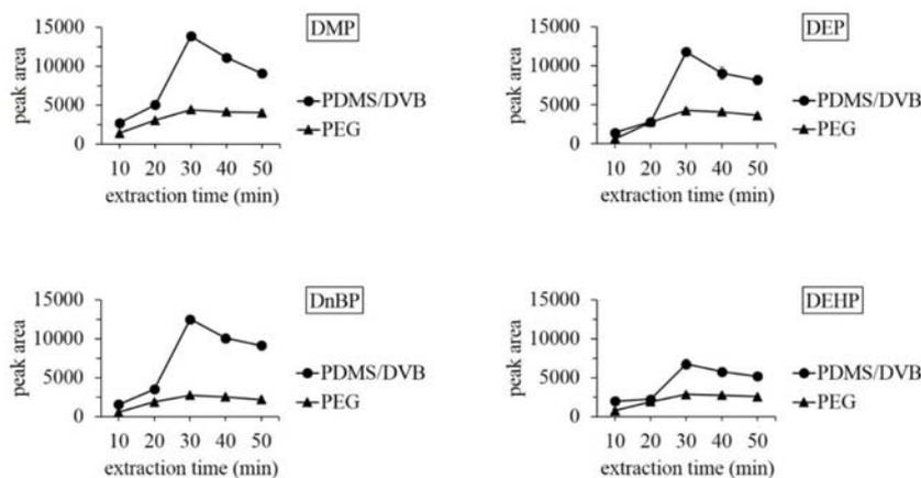
**Figure 2.** Effect of extraction time on HS-SPME of spiked  $200 \text{ ng mL}^{-1}$  of four phthalate esters in vegetable oil sample with extraction temperature of  $80 \text{ }^{\circ}\text{C}$ , desorption time of 10 min at  $200 \text{ }^{\circ}\text{C}$ .
