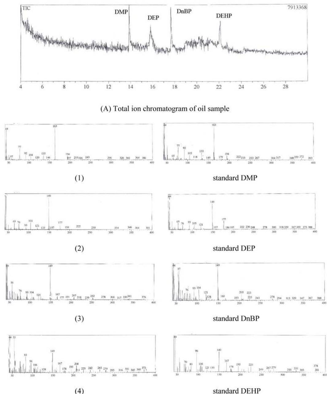
**Figure 5.** Total ion chromatogram of phthalate esters in sample (A) and mass spectra of compound 1,2,3,4, correspond to standard DMP, DEP, DnBP and DEHP, respectively.
