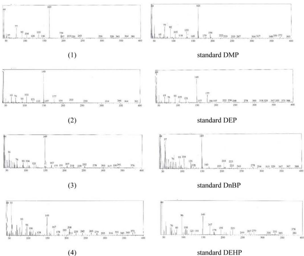
**Figure 5.** Total ion chromatogram of phthalate esters in sample (A) and mass spectra of compound 1,2,3,4, correspond to standard DMP, DEP, DnBP and DEHP, respectively.
