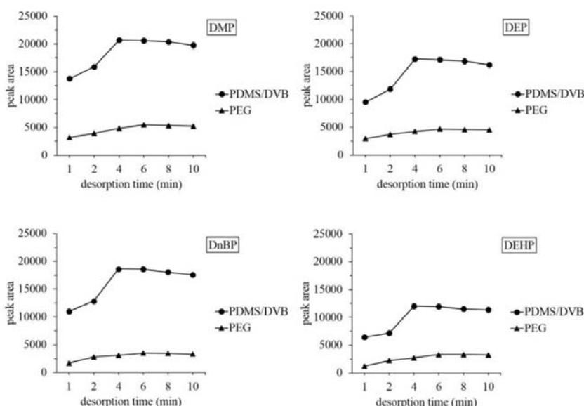
**Figure 3.** Effect of desorption time on HS-SPME of spiked  $200 \text{ ng mL}^{-1}$  of four phthalate esters in vegetable oil sample with extraction temperature of  $80 \text{ }^\circ\text{C}$ , extraction time of 30 min and desorption temperature of  $200 \text{ }^\circ\text{C}$ .
