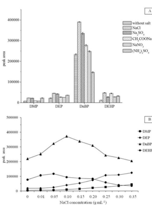
**Figure 4.** Effect of salt addition on HS-SPME in water matrix spiked sample using PDMS/DVB fiber with extraction temperature of 80 °C, extraction time of 30 min and desorption time 4 min at 200 °C. (A) effect of salt type, (B) effect of NaCl concentration.
