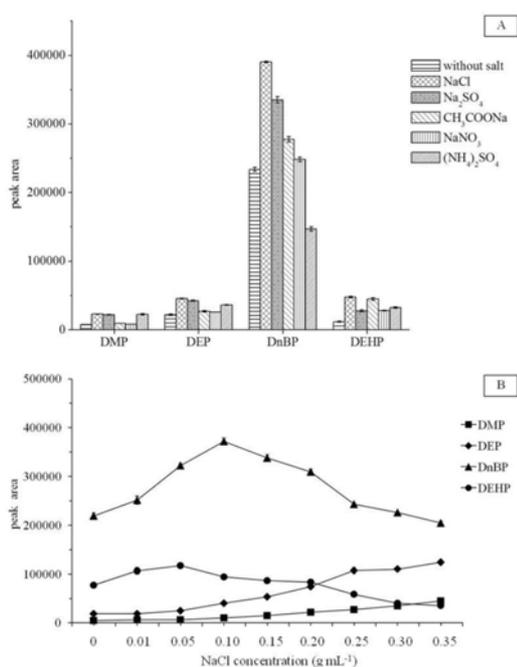
**Figure 4.** Effect of salt addition on HS-SPME in water matrix spiked sample using PDMS/DVB fiber with extraction temperature of 80 °C, extraction time of 30 min and desorption time 4 min at 200 °C. (A) effect of salt type, (B) effect of NaCl concentration.
