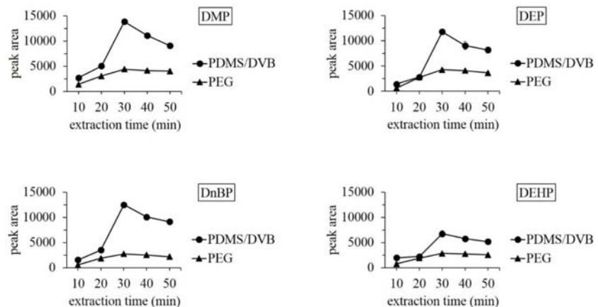
**Figure 2.** Effect of extraction time on HS-SPME of spiked 200 ng mL<sup>-1</sup> of four phthalate esters in vegetable oil sample with extraction temperature of 80 °C, desorption time of 10 min at 200 °C.
