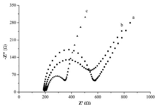
**Figure 5.** Nyquist plots of the different electrodes. a) SPCE, b) CNT/SPCE, and c) AuNPs-CNT/SPCE in 10 mM  $[\text{Fe}(\text{CN})_6]^{3-/4-}$  solution.
