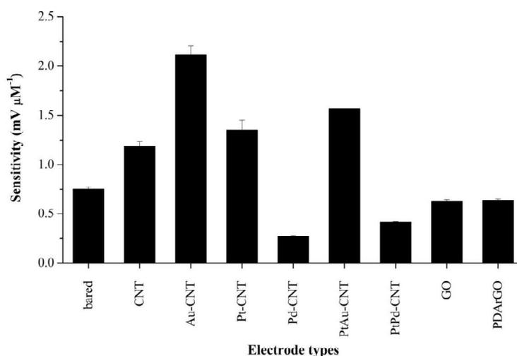
**Figure 2.** The sensitivity on the various modified electrodes for methyl dopa detection.
