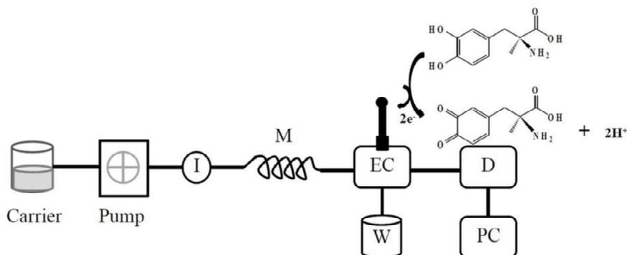
**Figure 1.** FI-amp system for determination of methyldopa.
