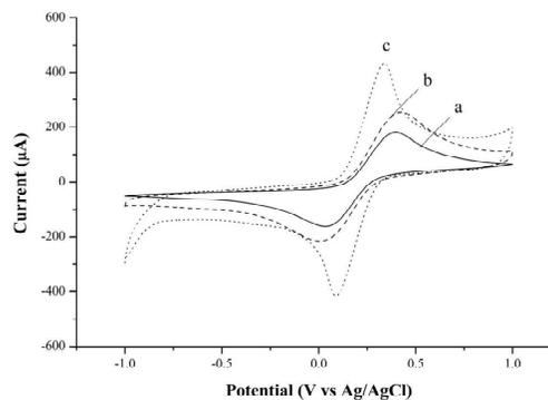
**Figure 4.** Cyclic voltammograms of a) SPCE, b) CNT/SPCE, and c) AuNPs-CNT/SPCE in 10 mM [Fe(CN)<sub>6</sub>]<sup>3-/4-</sup> solution.
