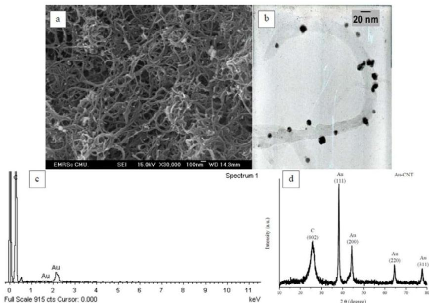
**Figure 3.** a) SEM image, b) TEM image, c) EDS spectrum, and d) XRD pattern of AuNPs-CNT.
