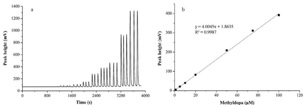
**Figure 6.** FIagram a) of signal response to methyl dopa concentration at 0.2, 0.5, 1, 5, 10, 20, 50, 75, 100, 250, and 500  $\mu\text{M}$  and b) the calibration graph of 0.2-100  $\mu\text{M}$ .
