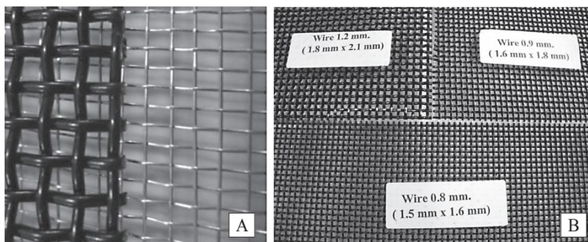
**Figure 2.** Steel mesh (16x16 openings) (left) and normal screen (14x17 openings) (right) (A) were used in the experiment; and 3 types of steel mesh (B) the 8x8 openings (upper left), 11x10.5 (upper right) and 16x16 openings (lower).
