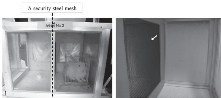
**Figure 1.** Mosquito preventive steel mesh test with a live rabbit host; the rabbit or mice were introduced in to a side of arena test and 200-400 mosquitoes were introduced into the other side of cage. The security steel mesh was put between rabbit side and mosquito side.
