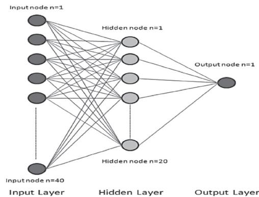
**Figure 2.** Architecture of the proposed neural network.
