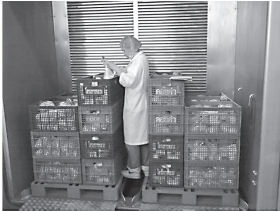
**Figure 2.** Arranging the plastic baskets in vacuum chamber.
