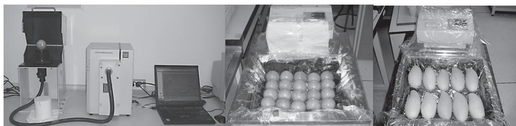
**Figure 1.** Measurement of NIR spectrum of fruit by using (a) NIRSystem6500 obtained with fiber optic probe (b) temperature control unit of fruit at 25°C.
