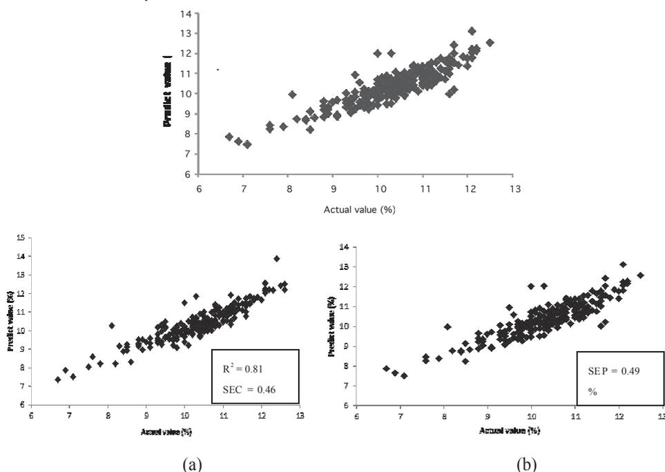
**Figure 4.** Plot of actual and predicted total soluble solid of strawberry fruit in (a) calibration set and (b) prediction set.
