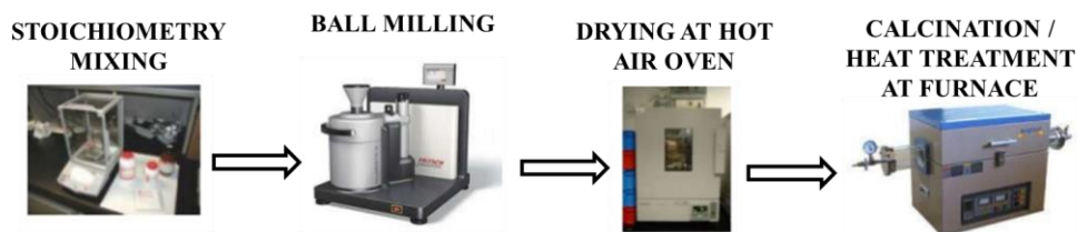
Figure 3. Pictorial representation of solid-state reaction method
