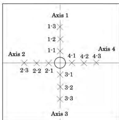
Figure 4 Hardness measuring positions (not to scale)
