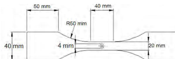
**Figure 3** Shape and dimensions of fatigue test specimen with a 4-mm diameter hole
