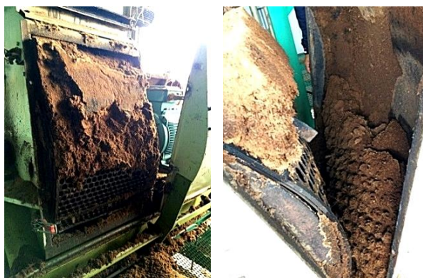
Figure 5 Jamming of crushed bark between the screen and the cover
