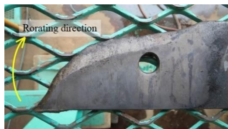
Figure 10 Corresponding abrasive directions with shaft rotating direction.
