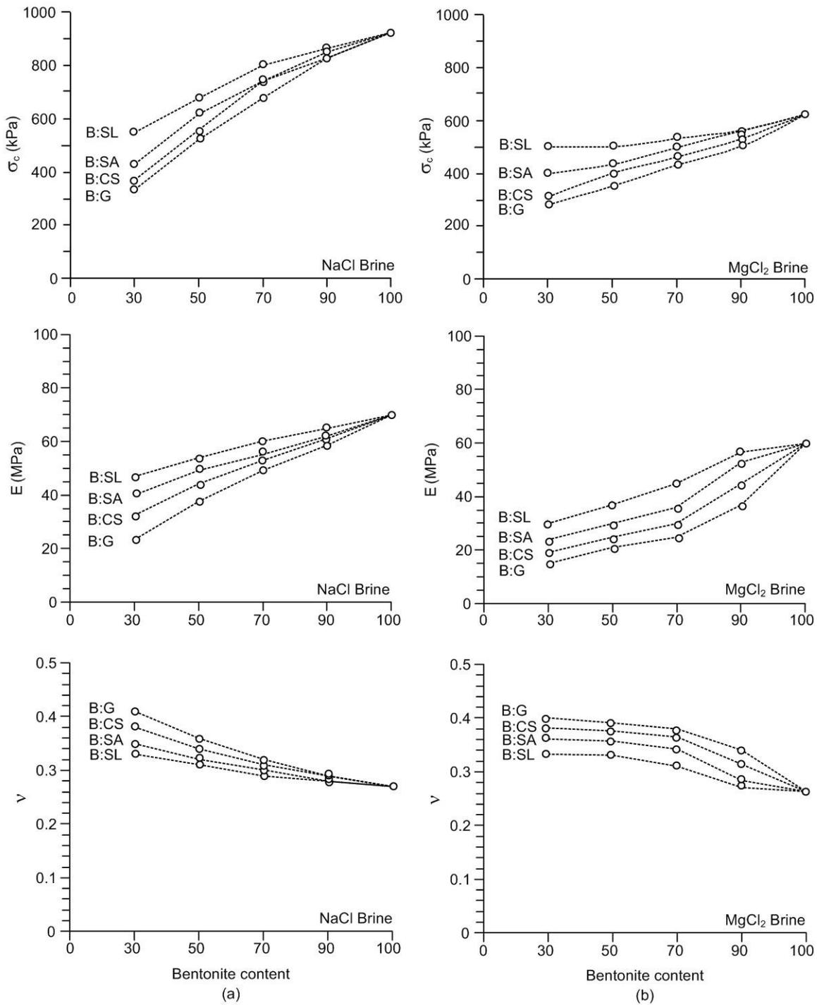
**Figure 5** Compressive strengths, Elastic moduli and Poisson's ratios as a function of bentonite content mixed with NaCl brine (a) and with MgCl<sub>2</sub> brine (b)
