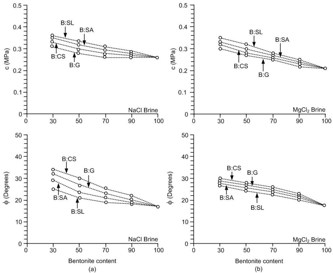
**Figure 4** Cohesions and friction angle as a function of bentonite content mixed with NaCl brine (a) and with MgCl<sub>2</sub> brine (b)
