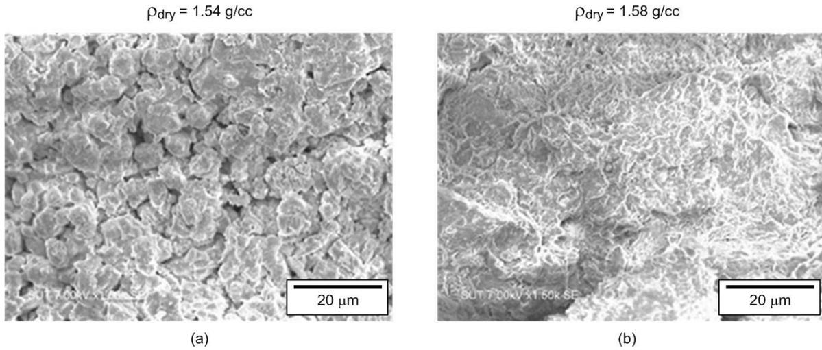
**Figure 3** SEM images of compacted pure bentonite mixed with NaCl (a) and MgCl<sub>2</sub> (b) brines
