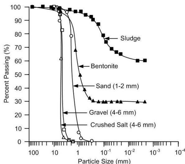
**Figure 1** Particle size distributions of tested materials
