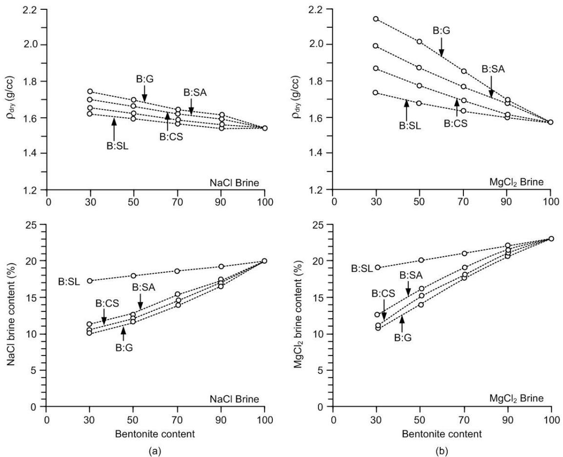
**Figure 2** Maximum dry densities and optimum brine contents as a function of bentonite content mixed with NaCl brine (a) and with MgCl<sub>2</sub> brine (b)
