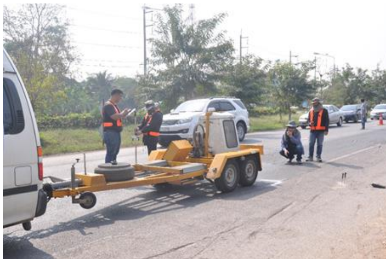
Figure 1 Dynatest Model 8000 Falling Weight Deflectometer (FWD) from Denmark.
