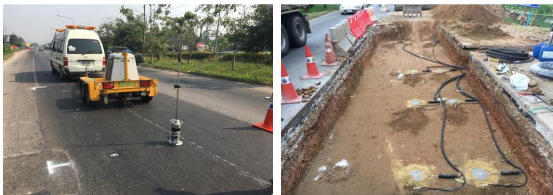
Figure 5 FWD measurement data and field measurement data from embedded instrumentation.
