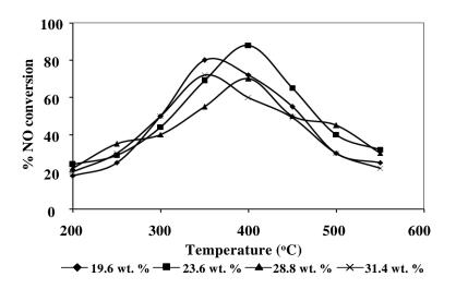
Figure 3. NO conversion profiles of monolith catalysts with various washcoat loadings. (Reaction conditions: 900 ppm NO, 2000 ppm i- $C_4H_{10}$ , 3 v %  $O_2$  and  $N_2$  as balance).
