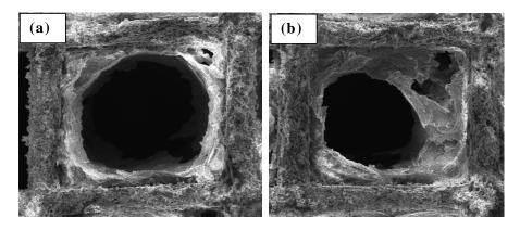
Figure 2. Typical images of the monolith cells when loaded with (a) 19.6 wt. % and, (b) 31.4 wt. % of Cu-Zn/ZSM-5.
