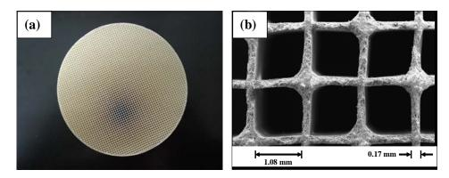
Figure 1. Picture of the ceramic monolith substrate used (a) and enlarged image of the cells (b).
