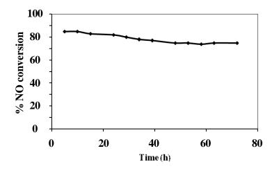
Figure 4. Stability of 23.6 wt. % Cu-Zn/ZSM-5 monolithic catalyst over long time on stream. (Reaction condition: 900 ppm NO, 2,000 ppm i- $C_4H_{10}$ , 3 v %  $O_2$  and  $N_2$  as balance and 400 °C).
