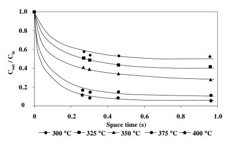
Figure 5. Dimensionless concentration of NO in the outlet as a function of space time at different reaction temperatures. (Reaction condition: 900 ppm NO, 2,000 ppm i-C<sub>4</sub>H<sub>10</sub>, 3 v % O<sub>2</sub> and N<sub>2</sub> as balance).
