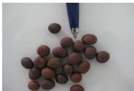
Figure 1. Image of commercial ceramic beads with the average diameter of ca. 5 mm.
