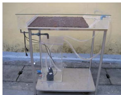
Figure 2. (a) schematic diagram and (b) real image of the pilot-scale supply water treatment system under natural sunlight with capacity of 2 m 3 /day.
