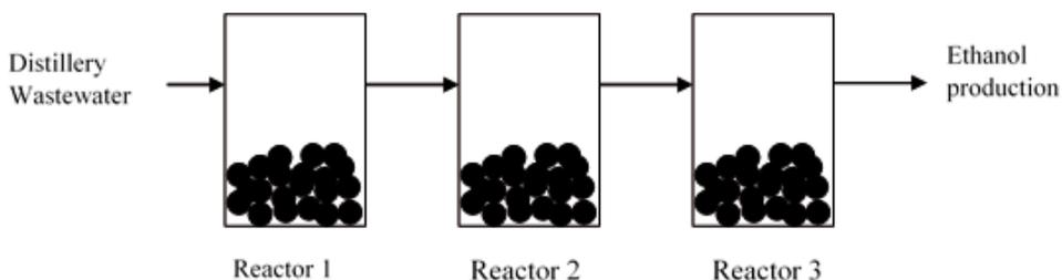
**Figure 2.** Schematic diagram of three reactors connected in series under anaerobic condition
