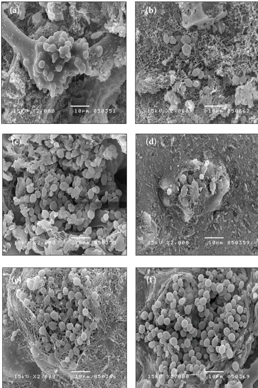
**Figure 5.** Electronic photomicroscope with magnification X2,000 of immobilized *S. cerevisiae* beads at cell concentration of 50% (v/v): (a) outer surface, (b) inner surface bead at PVA:POFA 10:1; (c) outer surface, (d) inner surface bead at PVA:POFA 10:2; (e) outer surface, (f) inner surface bead at PVA:POFA 10:3
