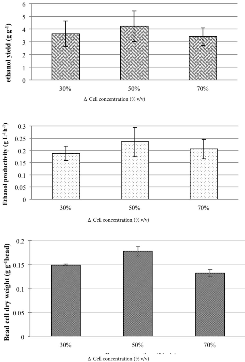
**Figure 3.** Ethanol yield, ethanol productivity, and bead cell dry weight, at HRT 24 h and PVA:POFA of 10:3 in batch reactor ( $p < 0.05$ ,  $N = 12$ )
