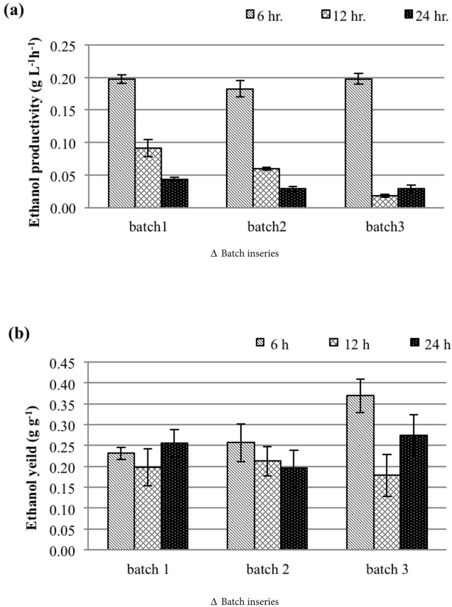
**Figure 7.** Ethanol productivity and ethanol yield at HRTs of 6, 12, and 24 hours under batch in series ( $p < 0.05$ ,  $N = 12$ )
