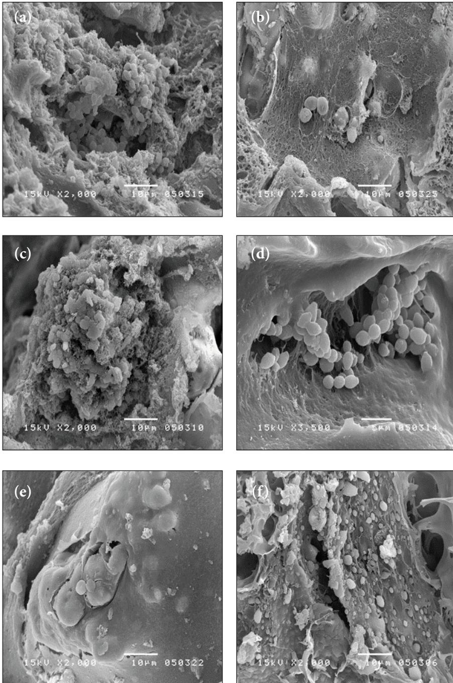
**Figure 4.** Electronic photomicroscope with magnification X2,000 of immobilized *S. cerevisiae* beads: (a) outer surface, (b) inner surface bead at cell concentration of 30% (v/v); (c) outer surface, (d) inner surface bead at cell concentration of 50% (v/v); (e) outer surface, (f) inner surface bead at cell concentration of 70% (v/v)
