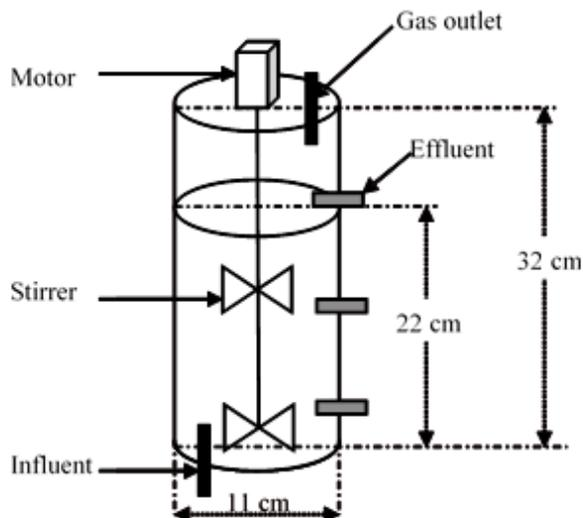
**Figure 1.** A schematic drawing of the experimental unit dimension
