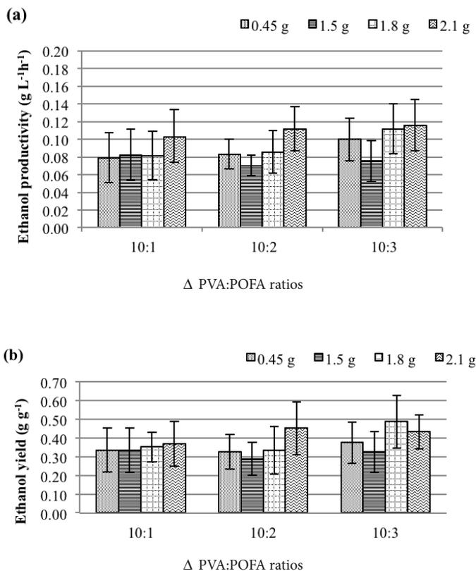
**Figure 6.** Ethanol productivity and yield as a function of initial cell dry weight of 0.45 g, 1.5 g, 1.8 g and 2.1 g under PVA: POFA ratios of 10:1, 10:2 and 10:3 ( $p < 0.05$ ,  $N = 12$ )
