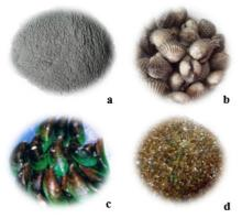
Figure 1. Raw materials (waste from Si Chang island): (a) cement waste, (b) cockle seashell waste, (c) mussel seashell waste, and (d) glass waste
