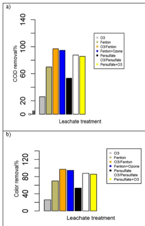
Figure 2. Showing the behaviour of selected treatment on a) COD removal and b) Color removal.
