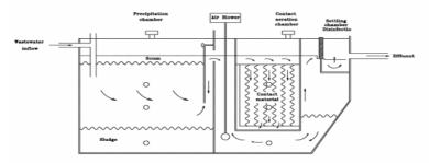
Figure 1. Schematic diagram of compact biological unit system (BCU).
