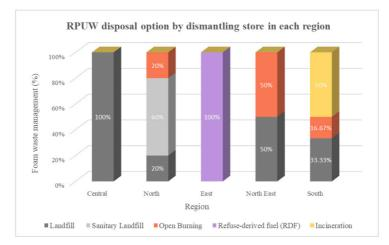
Figure 2. The rigid polyurethane foam wastes management in each region
