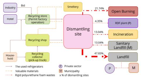
Figure 3. Route of rigid polyurethane foam wastes disposal in Thailand
