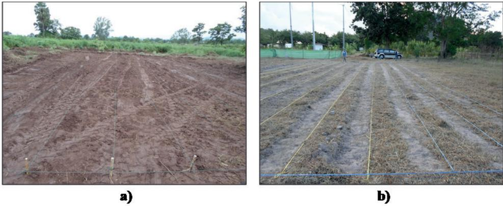
**Figure 3.** View of the two experimental sites with the GPR survey lines marked on the ground. (a) Loamy (to clay loam at 30 cm) soil site at Saraburi province and (b) loamy sand soil site at Petchaburi province.
