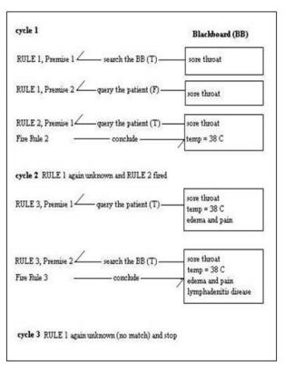
Fig.11: Example of Interactive Forward Chaining Processing
