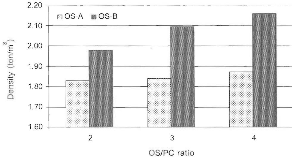
Figure 1. Relation of density of OS-A and OS-B concrete blocks against OS/PC ratio
