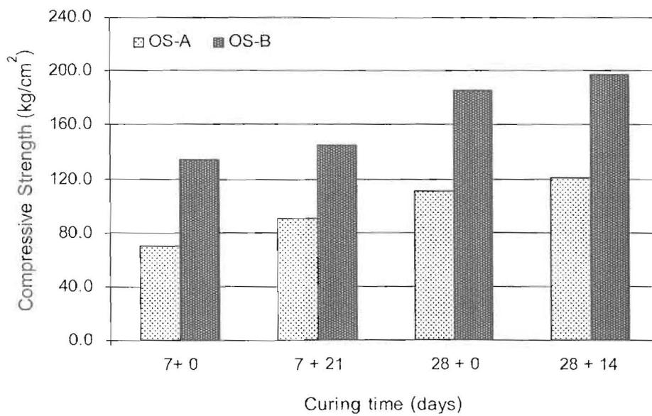
Figure 5. Relation of compressive strengths of OS-A and OS-B concrete blocks against curing time
