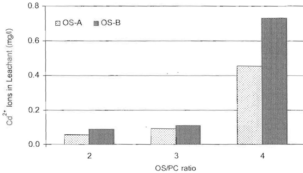
Figure 3. Relation of Cd<sup>2+</sup> in leachant of OS-A and OS-B concrete blocks against OS/PC ratio
