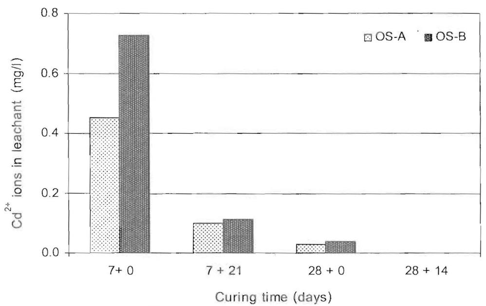
Figure 6. Relation of Cd<sup>2+</sup> Ions in leachant of OS-A and OS-B concrete blocks against curing time
