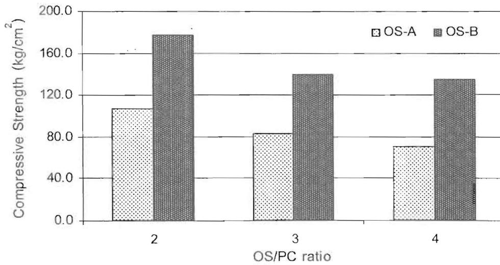
Figure 2. Relation of compressive strengths of OS-A and OS-B concrete blocks against OS/PC ratio
