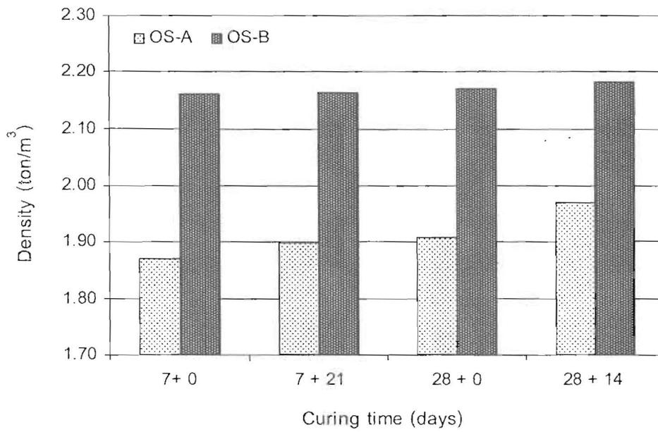
Figure 4. Relation of density of OS-A and OS-B concrete blocks against curing time
