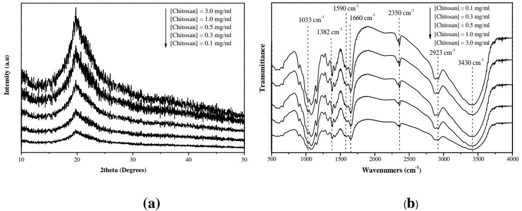
**Figure 1** Chitosan characterisation: (a) XRD pattern of chitosan at different concentrations; (b) FTIR spectra of chitosan nanoparticles at different concentrations.
