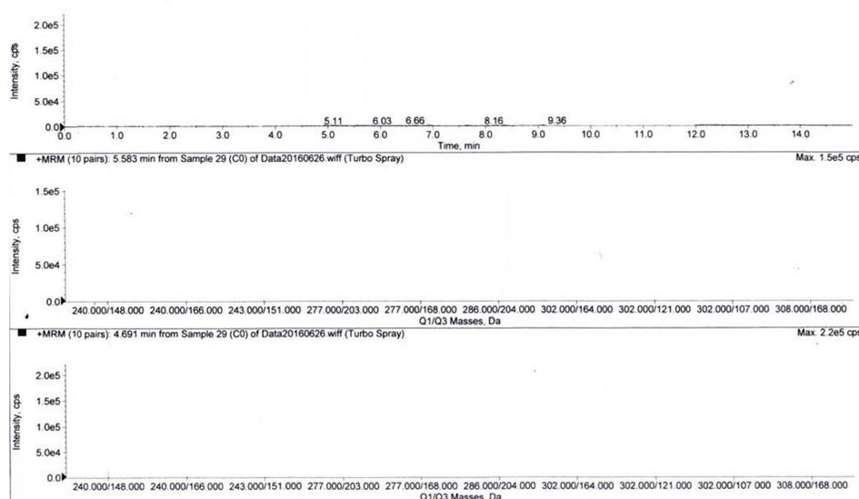
Figure 1. Typical ion chromatograms of extracts from blank plasma sample
