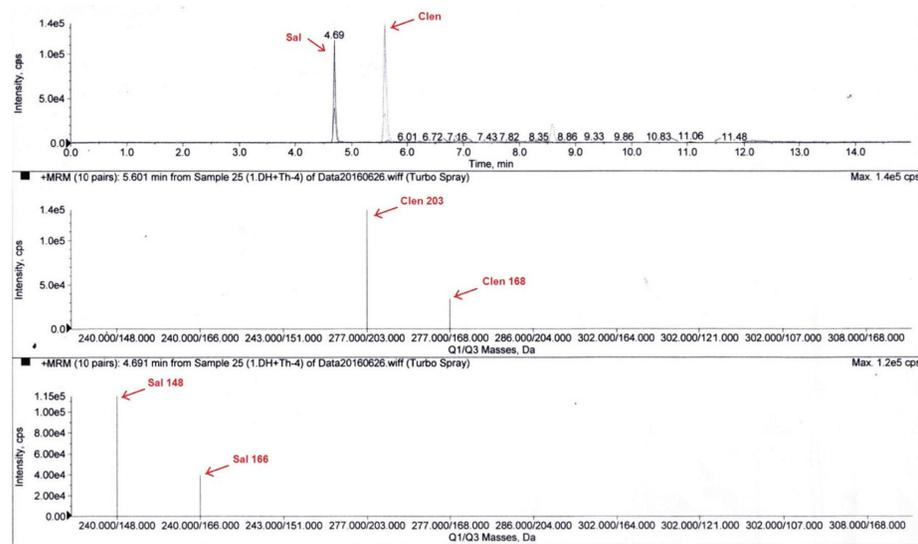
Figure 3. Typical ion chromatograms of standards of SAL (9 ppb) and CLEN (3 ppb)
