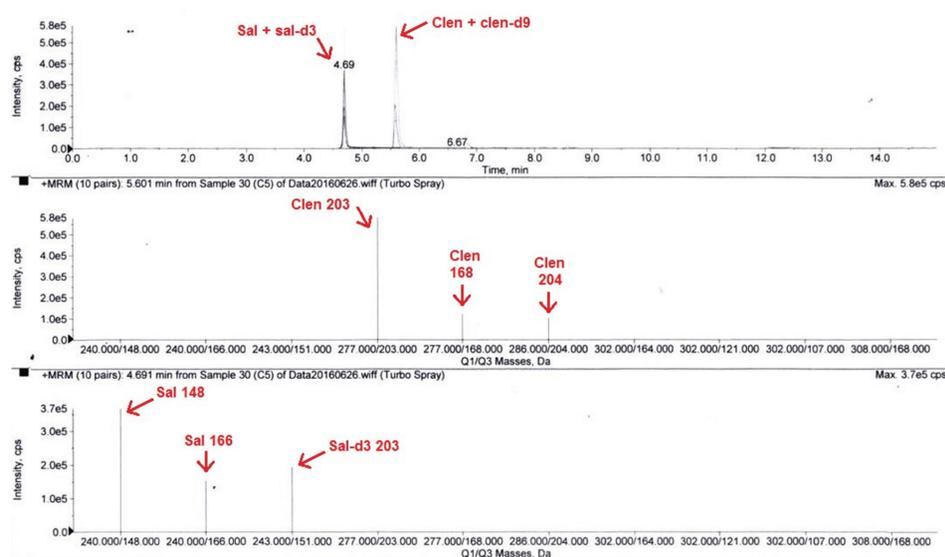
Figure 2. Typical ion chromatograms of extracts from plasma sample fortified with SAL (9 ppb), CLEN (3 ppb), SAL-d3 (2 ppb) and CLEN-d9 (1 ppb)
