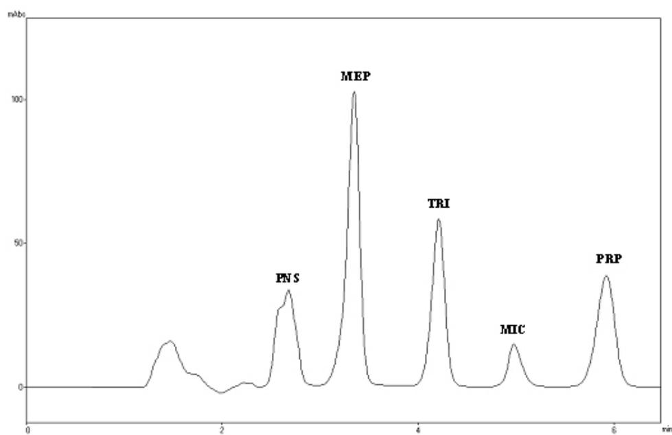
**Figure 3.** A typical chromatogram of a standard mixture of MIC, TRI, MEP, PRP and PNS. Condition: column: symmetry C8; 150 x 4.6 mm i.d., 5  $\mu$ m; mobile phase: ACN: 5 mM TCA in 0.05 % PA (48 : 52, % v/v); flow rate: 0.9 mL/min; UV detector: 264 nm.
