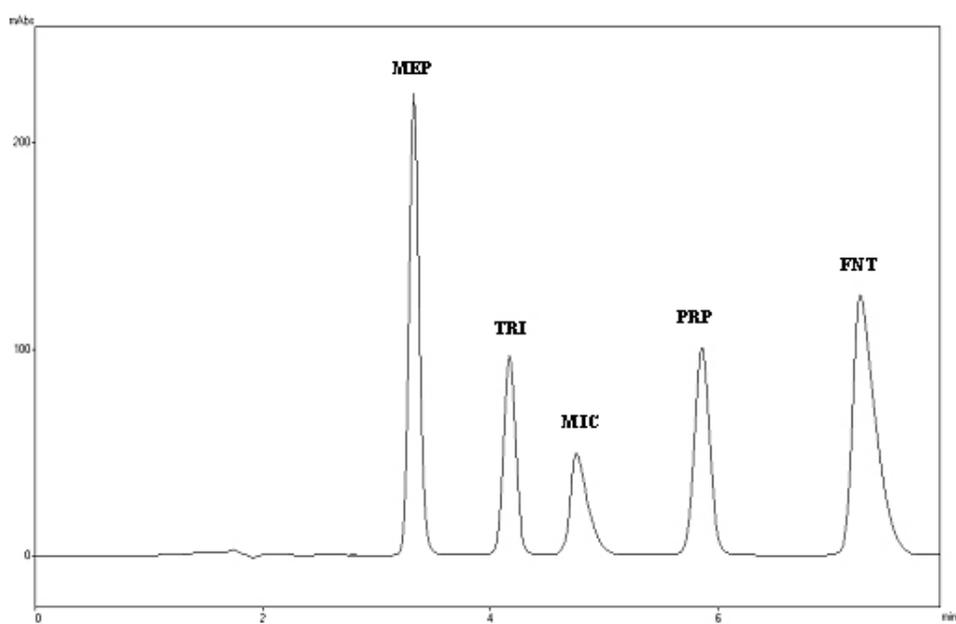
**Figure 4.** A typical chromatogram of a standard mixture of MIC, TRI, MEP, PRP and FNT. Condition: column: symmetry C8; 150 x 4.6 mm i.d., 5  $\mu$ m; mobile phase: ACN : 5 mM TCA in 0.05 % PA (48 : 52; % v/v); flow rate: 0.9 mL/min; UV detector: 264 nm.
