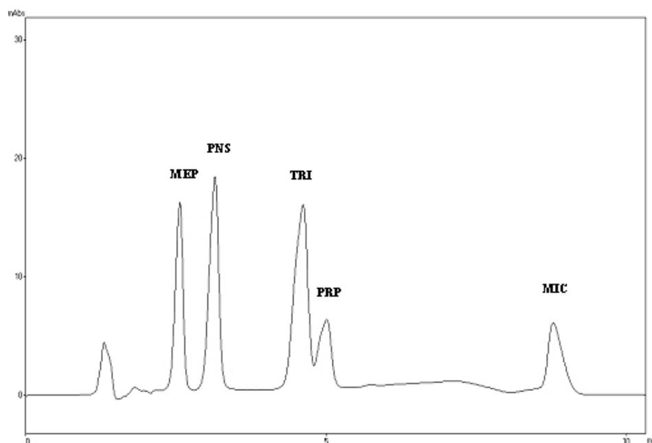
**Figure 2.** A typical chromatogram of a standard mixture of MIC, TRI, MEP, PRP and PNS. Condition: column: symmetry C18; 150 x 4.6 mm i.d., 5  $\mu$ m; mobile phase: MeOH / ACN / 5 mM trichloroacetic acid in 0.05 % phosphoric acid (30 / 30 / 40 ; % v/v/v); flow rate: 1 mL/min; UV detector: 264 nm.
