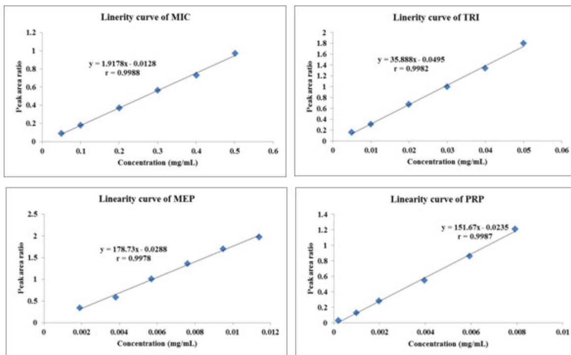
Figure 5. Calibration curves of (A) MIC, (B) TRI, (C) MEP and (D) PRP.
