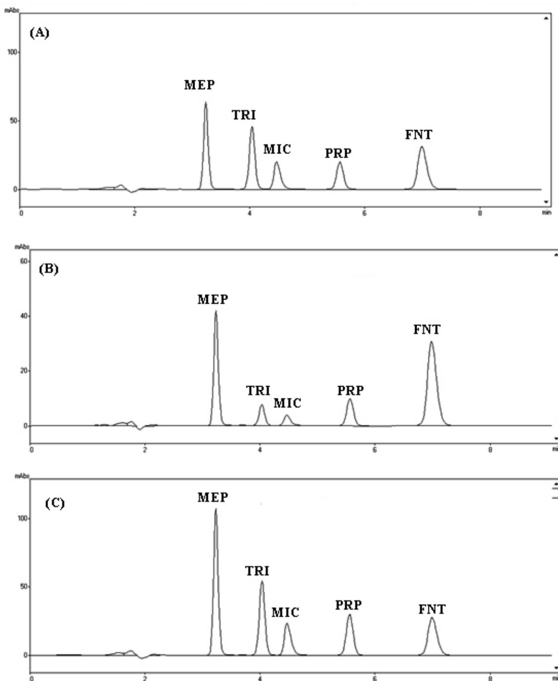
**Figure 6.** Chromatograms of (a) standard mixture solution; (b) cream solution; (c) standard mixture spiked cream solution. Condition: column: symmetry C8; 150 x 4.6 mm i.d., 5  $\mu$ m; mobile phase: ACN : 5 mM TCA in 0.05 % PA (48 : 52; % v/v); flow rate: 0.9 mL/min; UV detector: 264 nm.
