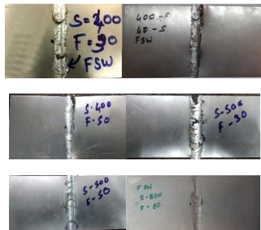
Figure 5. Defective welded joints made in air at lower tool traversing speed and higher tool rotational speeds
