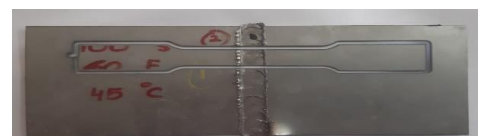
Figure 4. Specimen cut for tensile testing
