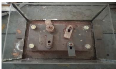
Figure 1. Setup for underwater FSW
