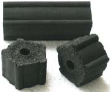
Figure 9. Schematic of Extruded fuel from the experiments.
