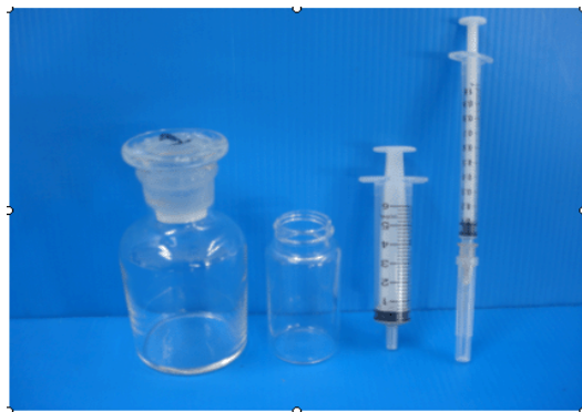
Figure 1. Materials for the self-prepared test kit for outdoor dissolved oxygen determination.
