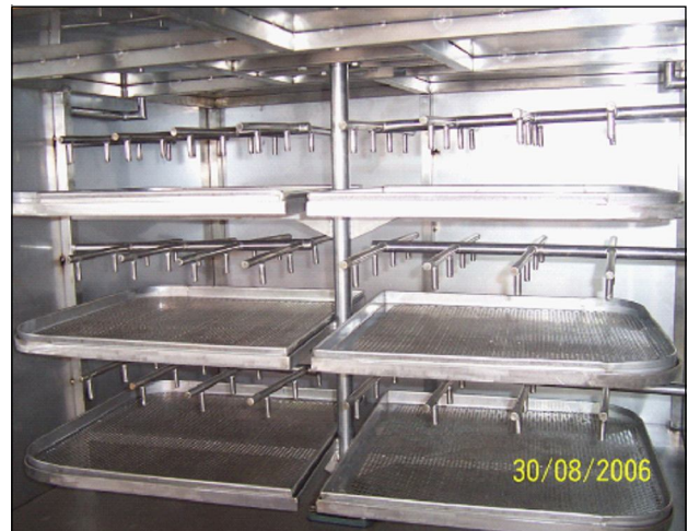
Figure 6. Pilot-scale impingement dryer showing impinging nozzles and drying trays.
