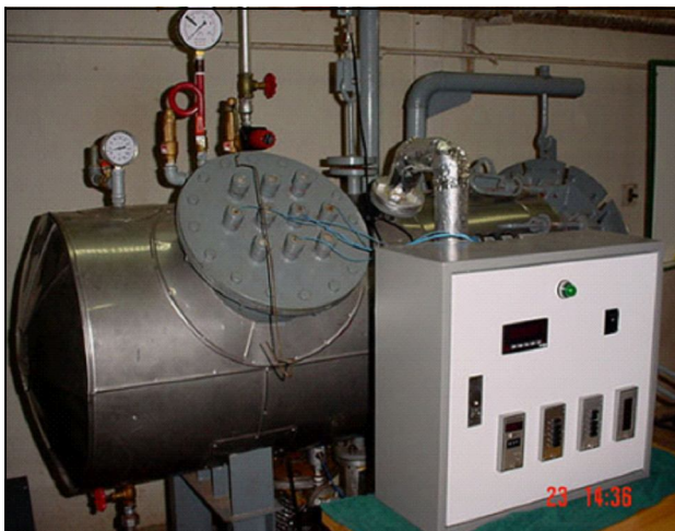
Figure 4. Air-impingement dryer used in the lab-scale experiment.
