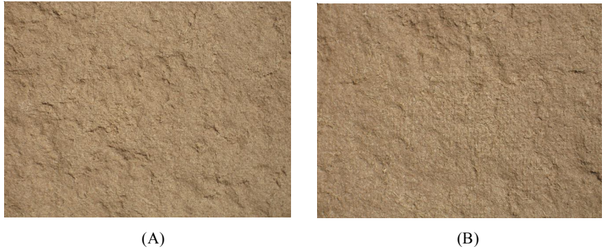
Figure 2. Surfaces of insulation boards made from empty fruit bunches (A) and oil palm fronds (B).
