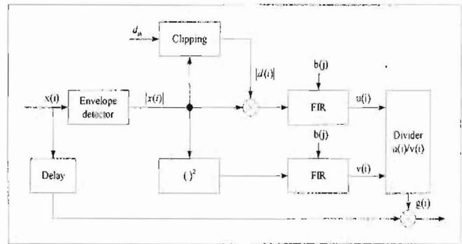
Figure 3. Block diagram of conventional APPR
