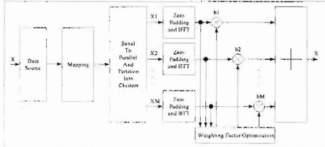
Figure 2. Block diagram of the conventional PTS technique.
