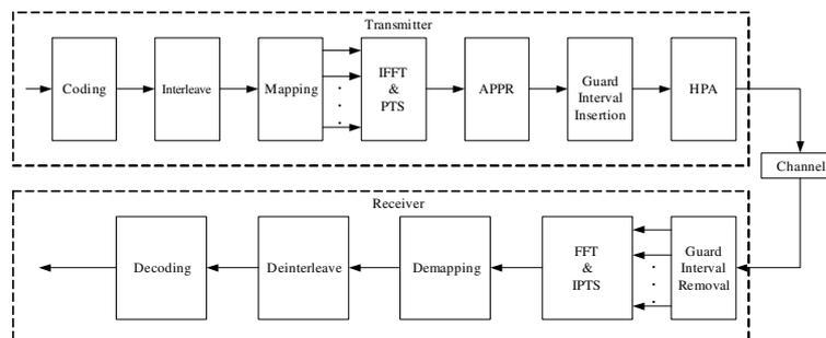
Figure 5. Block diagram of the total system used for the simulation
