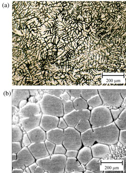
Figure 10. Microstructure of (a) liquid Al-4.4%Cu and (b) semi-solid Al-4.4%Cu (both 50x).
