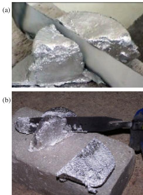
Figure 8. Cream-like behavior of semi-solid metals (a) A356 and (b) Al-4.4%Cu, demonstrated by a knife-cutting test.
