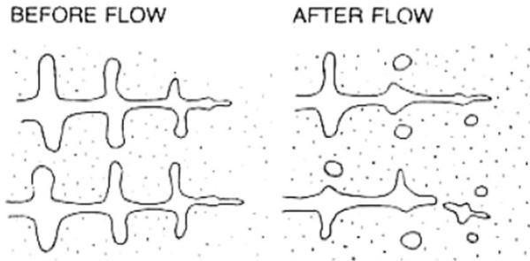
Figure 4. Schematic of dendrite multiplication (Flemings, 1971).
