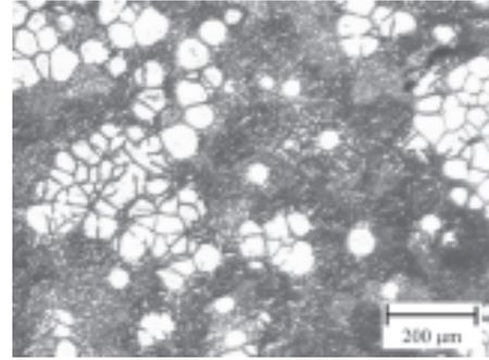
Figure 12. Microstructure of semi-solid Al-4.4%Cu after 20 seconds of gas bubbling and quenched in water (50x).
