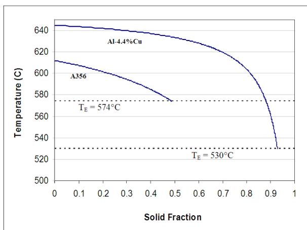
Figure 7. Solid fraction curves of the A356 and Al-4.4%Cu alloy. Dashed lines indicate the eutectic temperatures.
