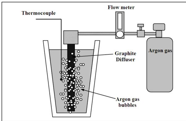
Figure 5. Schematic of the experimental setup used in this study, not to scale.
