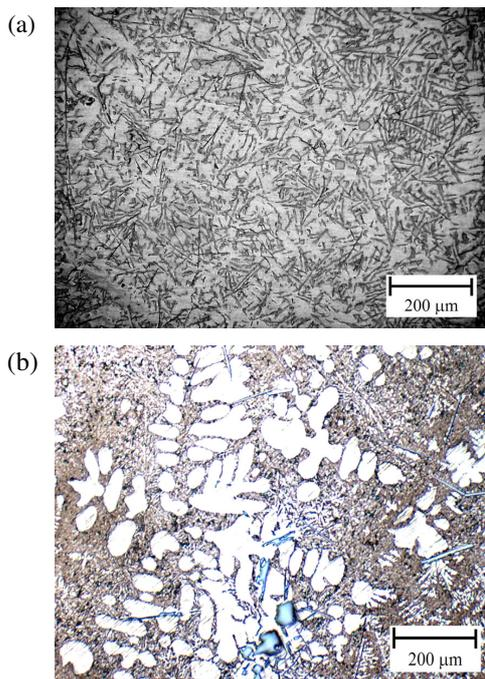
Figure 11. Microstructure of (a) liquid ADC12 and (b) semi-solid ADC12 after 20 seconds of gas bubbling (both 50x).
