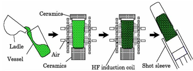
Figure 1. Process description of the NRC™ process (Courtesy of UBE Machineries).
