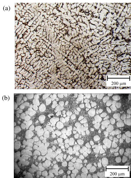
Figure 9. Microstructure of (a) liquid A356 and (b) semi-solid A356 (both 50x).
