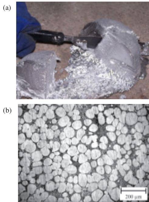
Figure 13. Results of the 2-kg A356 SSM processing: (a) knife-cutting test, (b) representative microstructure (50x).
