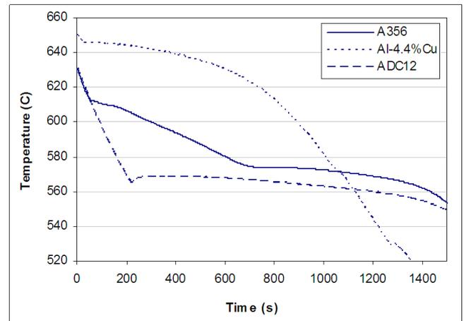
Figure 6. Cooling curves of the three aluminum alloys used in this study.
