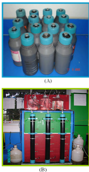
Figure 1. The 1-l bottles (A) and UASB reactors (B) used in this work.
