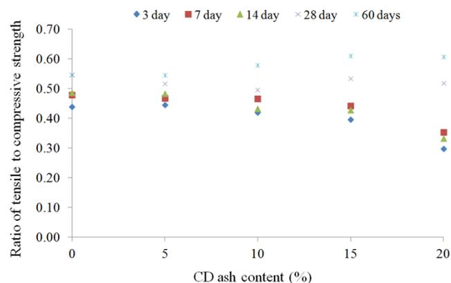
Figure 4. Ratio of tensile and compressive strength.
