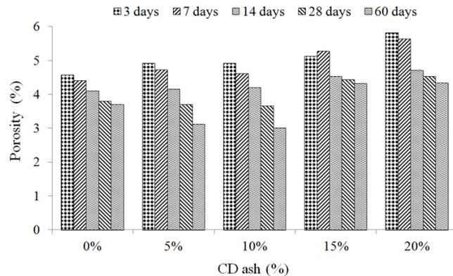
Figure 6. Porosity and content of CD ash.
