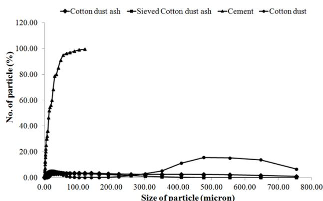
Figure 2. Particle size distribution of CD ash.
