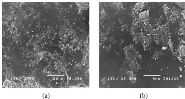
Figure 3. (a) SEM images of concrete mixed with CD ash (500x).
