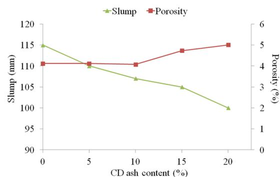
Figure 7. Relationship between slump and porosity of concrete mixed CD ash.
