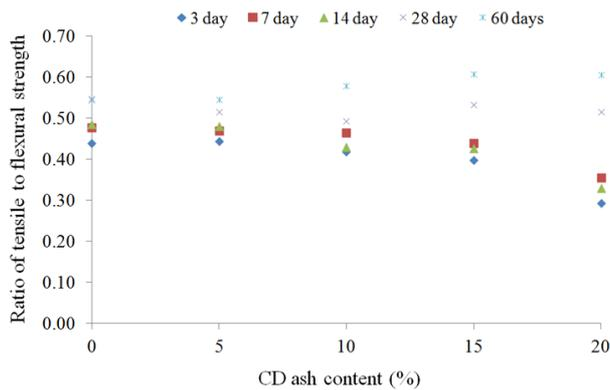
Figure 5. Ratio of tensile and flexural strength.
