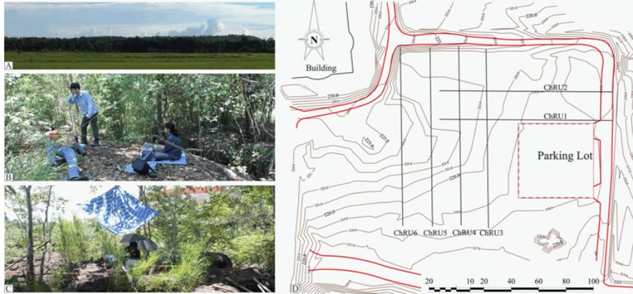
Figure 3. View of (A) the cuesta topography of the study area; views (B and C) along survey profiles illustrating the complex terrain consisting of large boulders and bedrocks on the surface; schematic plan view of location of the resistivity profiles ChRU1-6 (D).
