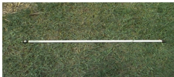
Figure 2. Quantum sensor for below canopy measurement of PAR.
