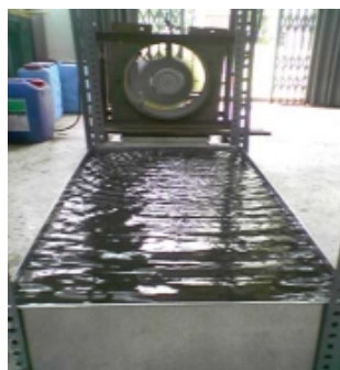
Figure 1. Pilot volatilization tank equipped with a wind generator system [Color figure can be viewed in the electronic version]
